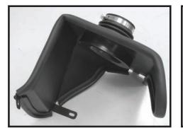
Step 5 Install the rubber bulb seal. Place the velocity stack adapter in the heat shield and install the supplied flex coupler making sure the coupler is pushed completely against the heat shield. Once the adapter and coupler are tight against the heat shield, tighten the clamp.
