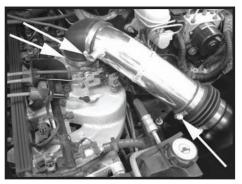
Step 10 Install the intake tube into the flex coupler and then install the 90° coupler to the intake tube and then position it onto the throttle body as shown. Once in desired position fasten it securely in place.
