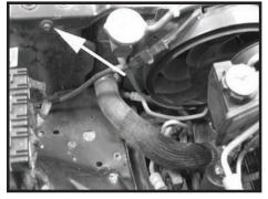
Step 7 Remove the bolt on the core support and this bolt will be reused in the next step.
