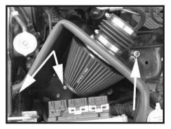
Step 8 Install the heat shield into the vehicle as shown by reusing the hardware from Step 4 and Step 7.
